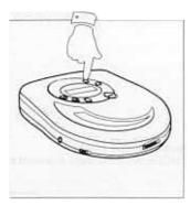
During stop, press PROG button until "PROG" flashes in LCD. The track number and playing order appears.
